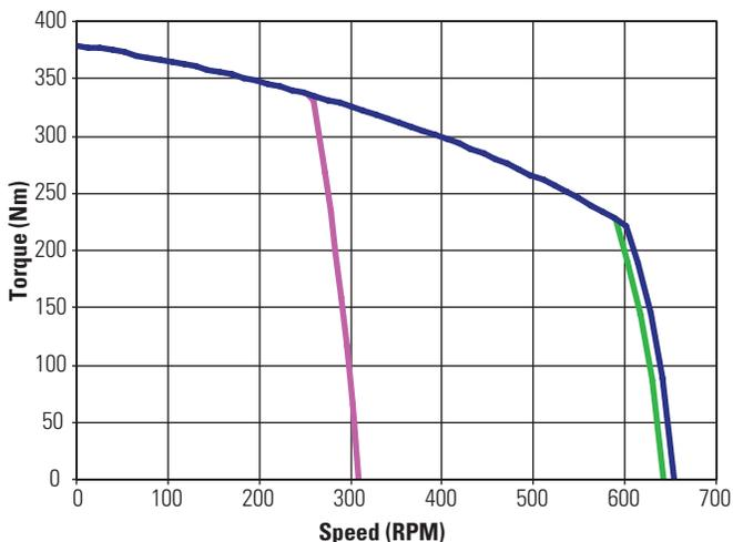
— A Winding-400 Vac — B Winding-480 Vac — C Winding-400 Vac
