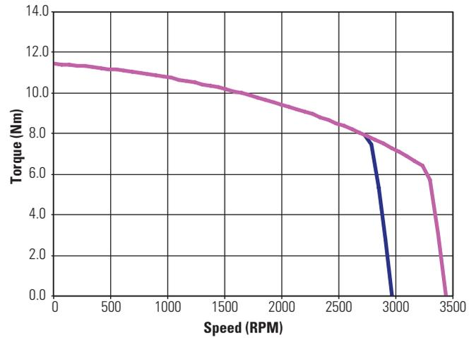
— A Winding-480 Vac / C Winding-400 Vac / D Winding-240 Vac
