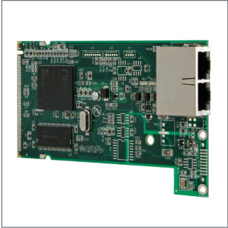
NETcore® X Industrial Ethernet APCI / MiniAPCI / MB1021 format
